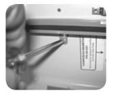
If the pins are flat, use a screwdriver to tap them out through the enclosure wall.
