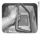
Make sure the frame is loose by pushing the right side down into the enclosure and pull the entire frame out of the enclosure by lifting the left side.
