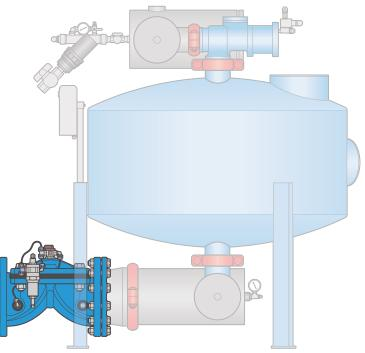
PRM valves automatically maintain the set upstream pressure for proper back wash by decreasing pressure and flow down stream. They also allow for manual operation.
