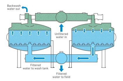
The new JAIN under drain has very high uniformity with no downward jetting. High uniformity decreases back wash time, saves water, energy and decreases maintenance. Downward jetting can compromise tank coating reducing tank life.
